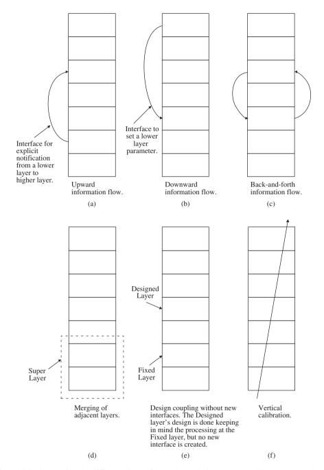
Figure 6.1 Illustrating the different kinds of cross-layer design proposals. The rectangular boxes represent the protocol layers
